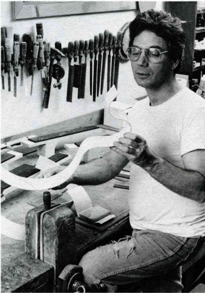
D'Aquisto checks side bending accuracy before gluing up rims.
